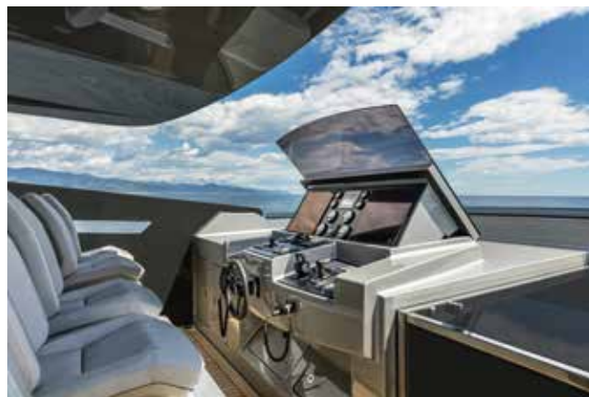
The flybridge has six pilot seats at the helm, where the screens and windshield can fold down
